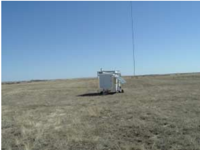
Figure 1 Installation of an ART, LLC model VT-1 sodar at a site in southern Saskatchewan, Canada.
